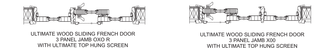
ULTIMATE WOOD SLIDING FRENCH DOOR 3 PANEL JAMB OXO R WITH ULTIMATE TOP HUNG SCREEN ULTIMATE WOOD SLIDING FRENCH DOOR 3 PANEL JAMB X00 WITH ULTIMATE TOP HUNG SCREEN
